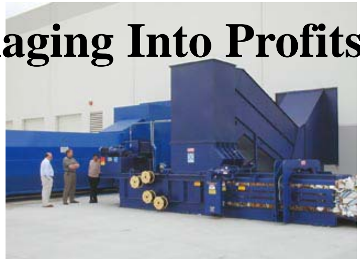
An automatic tie baler accepts whole boxes and then compacts and bales them in just seconds.
